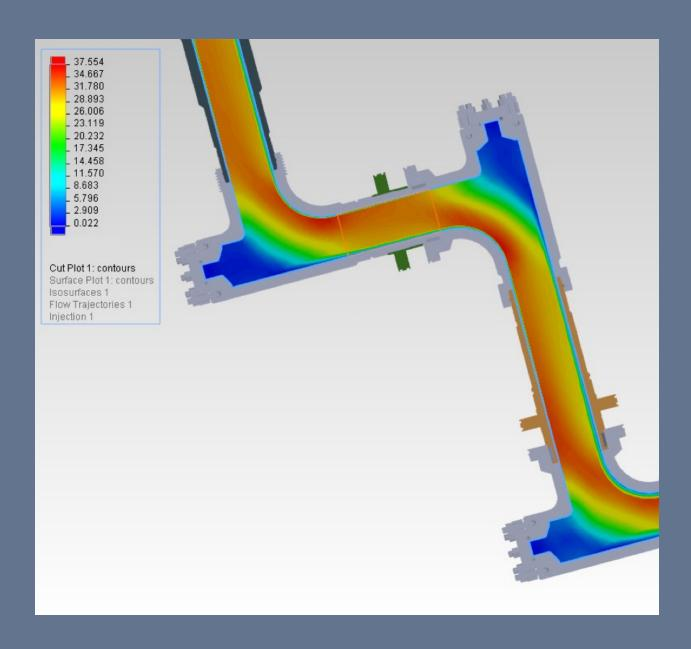
FHE dynamic flow iron optimizes media flow path to eliminate dangerous "dead spots" and drastically reduces erosion velocity which decrease erosion and adds significantly to the longevity of the flow iron. The internal diameter is 7" and can supply 130 barrels a minute.
