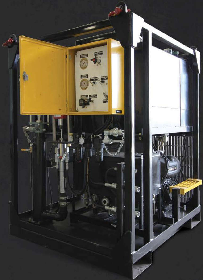
Dual 50-gallon grease tanks hold different grease viscosities for changing conditions.
