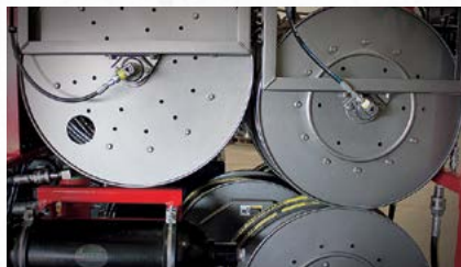
Hannay hydraulic and spring reels with adjustable speed.
