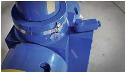
Swivel port for a gauge, valves, etc.
