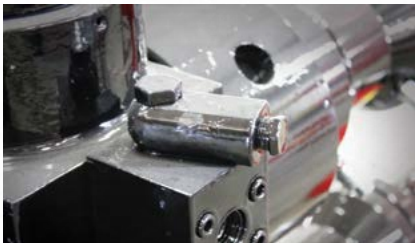
Swivel port for a gauge, valves, etc.
