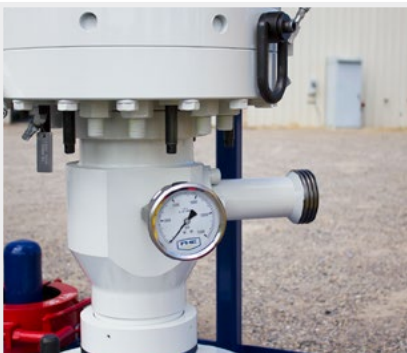
THE RIGLOCK REPLACES THE PUMP IN SUB WITH LARGE AUXILIARY PORT.
