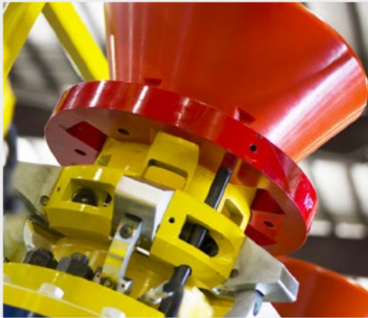
CAM LOCKS SECURE THE CONNECTION AND ARE REINFORCED WITH THE MECHANICAL RING LOCK.
