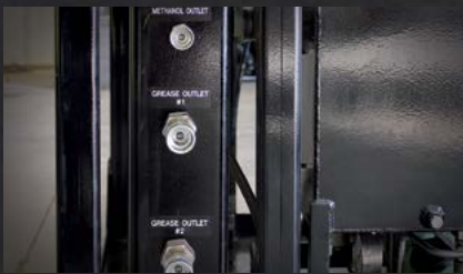
Quick connect bulkhead supply grease and methanol with quick connections.
