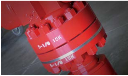
Flanged sub connections.
