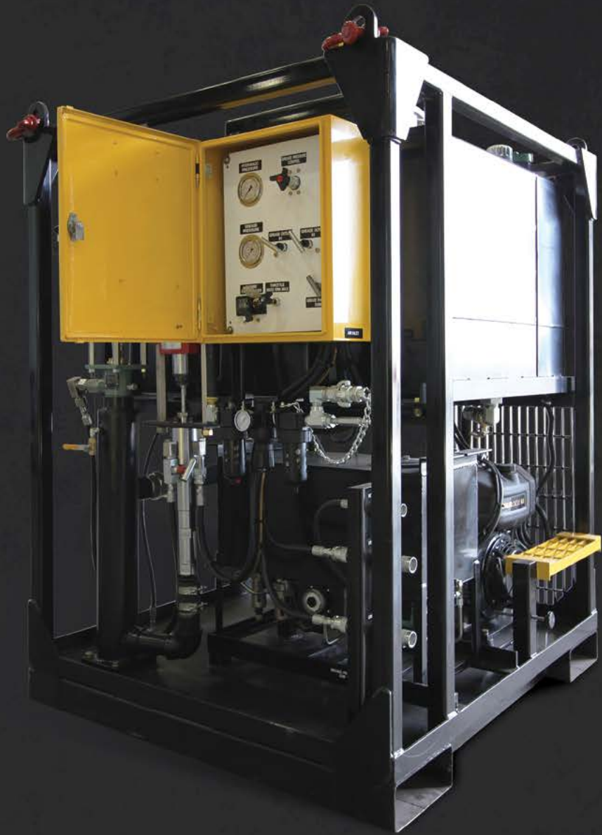
Dual 50-gallon grease tanks hold different grease viscosities for changing conditions.
