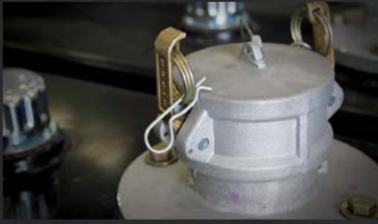
Dual 50-gallon grease tanks hold different grease viscosities for changing conditions.
