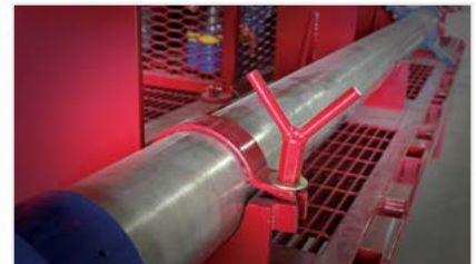
Secure lubricator rack protects the risers from damage during transportation and unloading.
