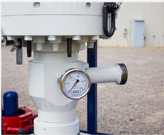
The Riglock® replaces the pump in sub with large auxiliary port.
