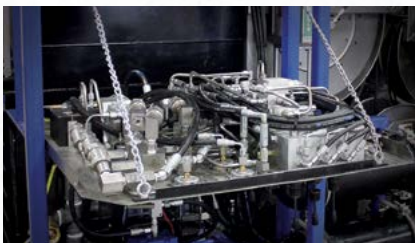
Fold-down control panel to easily access all hydraulic valves.
