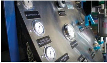
Fold-down control panel to easily access all hydraulic valves.
