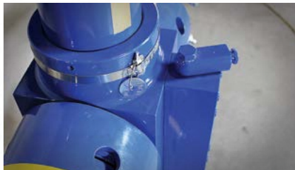
Swivel port for a gauge, valves, etc.
